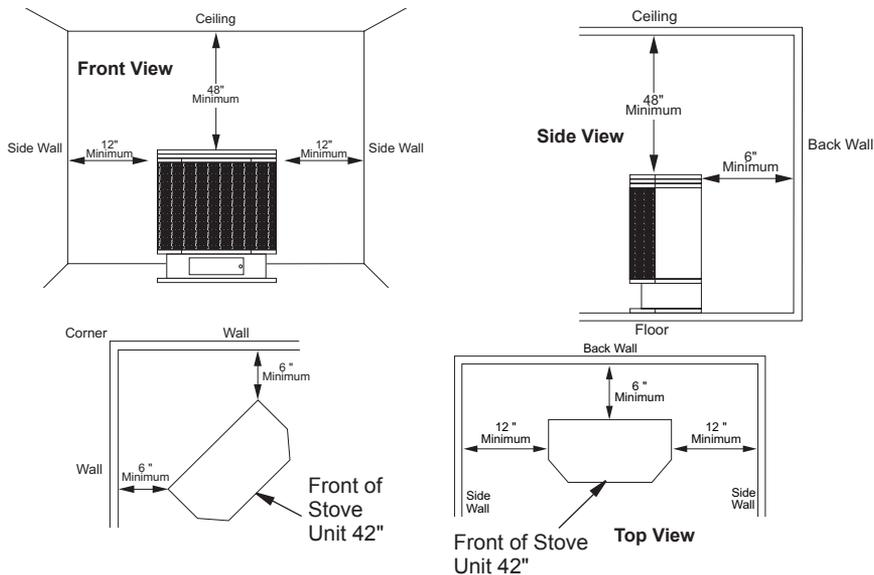
Figure 4 - Minimum Clearance to Walls and Ceiling
