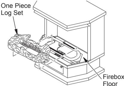
Figure 11 - Installing One-Piece Log Set
