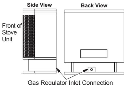
**Figure 5 - Gas Regulator Location and Gas Line Access Into Stove Cabinet**
