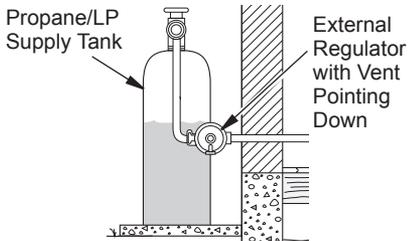
**Figure 6 - External Regulator With Vent Pointing Down**
