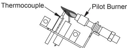
**Figure 21 - Correct Pilot Flame Pattern (Natural Gas Shown)**
