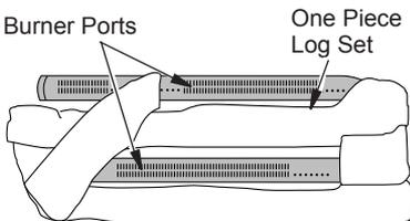
Figure 12 - Installing One-Piece Log set (Top View)
