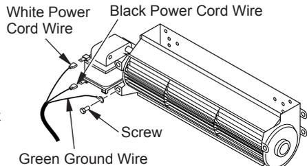
Figure 14 - Removing Wires from Blower
