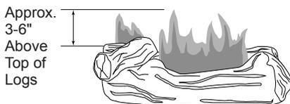
**Figure 23 - Correct Flame Pattern with Control Knob Set to High Flame**
