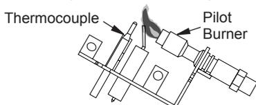
**Figure 22 - Incorrect Pilot Flame Pattern (Natural Gas Shown)**
