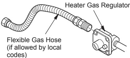
**Figure 11 - Attaching Flexible Gas Hose to Heater Gas Regulator (Variable Manually-Controlled and Thermostatically-Controlled Models Only)**
