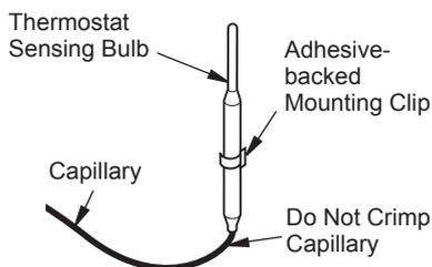
**Figure 51 - Positioning the Thermostat Sensing Bulb in the Vertical Position with the Capillary at the Bottom**
