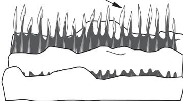
**Figure 42 - Incorrect Front Burner Flame Pattern**
