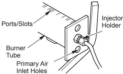
**Figure 43 - Injector Holder On Outlet Burner Tube**
