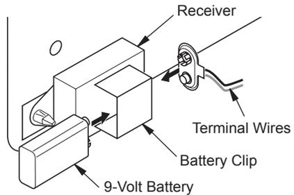
**Figure 24 - Installing Receiver on the Back of the Base**
