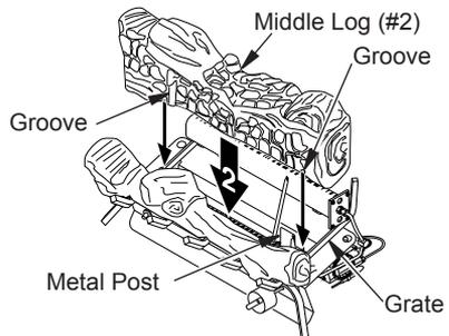
**Figure 27 - Installing Middle Log (#2)**
