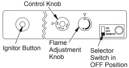
**Figure 33 - Control Knob and Ignitor Button Location**
