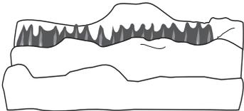
**Figure 41 - Correct Front Burner Flame Pattern**
