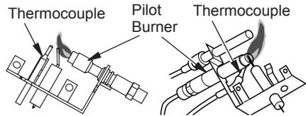
**Figure 40 - Incorrect Pilot Flame Pattern (Your pilot may vary from pilots shown)**
