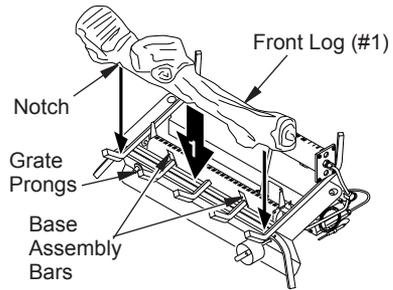
**Figure 26 - Installing Front Log (#1)**
