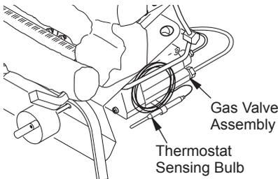
**Figure 45 - Location of Gas Valve Assembly and Thermostat Sensing Bulb**
