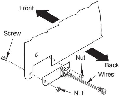
**Figure 21 - Switch Plate and Wiring Harness (Switch Plate and Orientation May Vary Depending On Model)**
