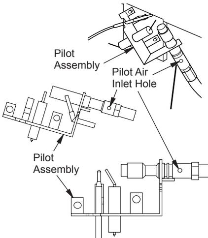
**Figure 44 - Pilot Inlet Air Hole (Your pilot may vary from pilots shown)**
