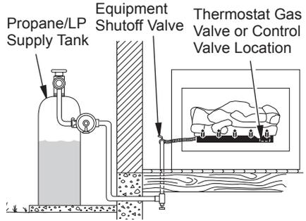
**Figure 19 - Checking Gas Joints (Propane/LP Only)**
