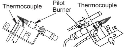
**Figure 39 - Correct Pilot Flame Pattern (Your pilot may vary from pilots shown)**
