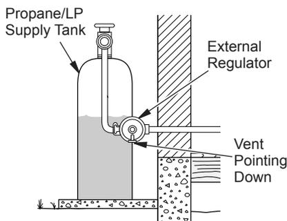
**Figure 15 - External Regulator With Vent Pointing Down**
