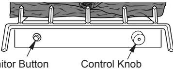
**Figure 31 - Control Knob and Ignitor Button Location**
