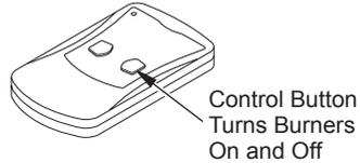
**Figure 37 - On/Off Hand-Held Remote Control Unit (HRC100)**
