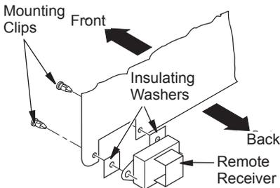
**Figure 22 - Installing Remote Receiver**
