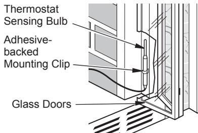
**Figure 50 - Installing Thermostat Sensing Bulb behind Glass Doors**
