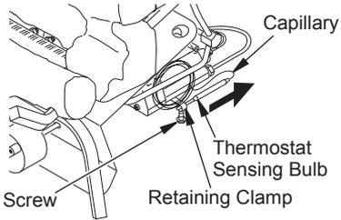
**Figure 47 - Removing Thermostat Sensing Bulb**
