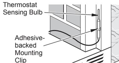
**Figure 49 - Locating Thermostat Sensing Bulb on Factory-built Metal Fireplace**
