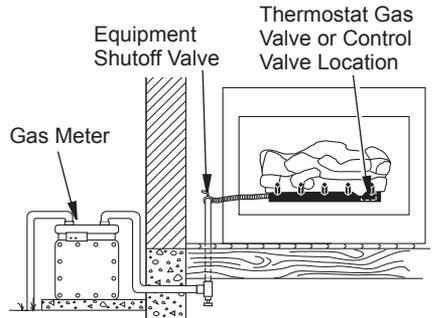
**Figure 20 - Checking Gas Joints (Natural Gas Only)**
