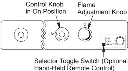
**Figure 36 - Setting the Selector Switch, Control Knob and Flame Adjustment Knob for Remote Operation**
