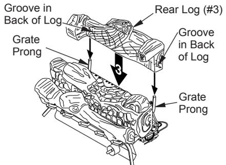
**Figure 28 - Installing Rear Log (#3)**
