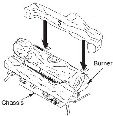
**Figure 28 - Installing Golden Oak 5-Piece Log Set - Log 3**
