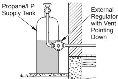
**Figure 15 - External Regulator With Vent Pointing Down**
