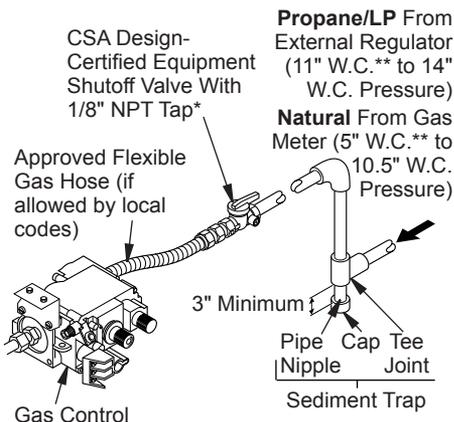
**Figure 17 - Gas Connection (Remote-Ready Models Only)**
