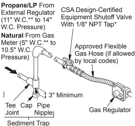
**Figure 16 - Gas Connection (Variable Manually-Controlled Models Only)**
