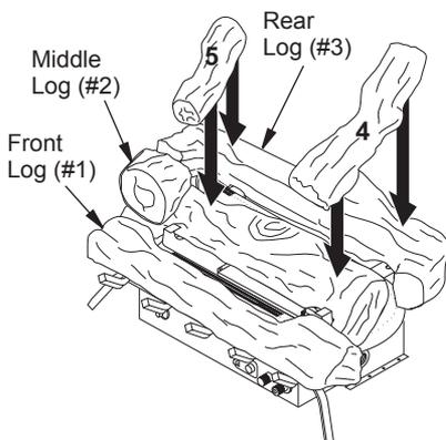
**Figure 29 - Installing Golden Oak 5-Piece Log Set - Logs 4 and 5**
