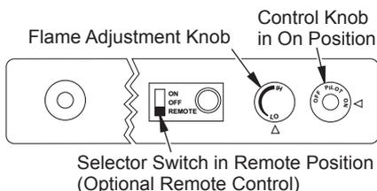
**Figure 35 - Setting the Selector Switch, Control Knob, and Flame Adjustment Knob for Hand-Held Remote Operation**
