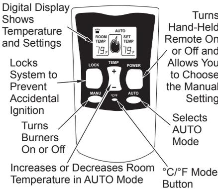
**Figure 37 - Thermostat Hand-Held Remote Control Unit (HRC200)**
