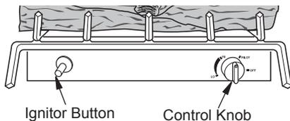
**Figure 30 - Control Knob and Ignitor Button Location**
