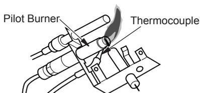
**Figure 39 - Incorrect Pilot Flame Pattern**
