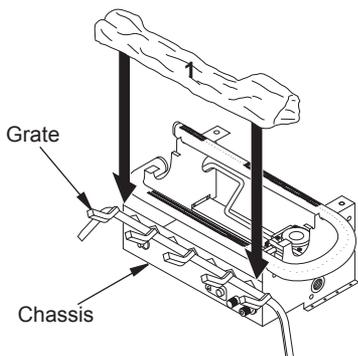
**Figure 26 - Installing Golden Oak 5-Piece Log Set - Log 1**
