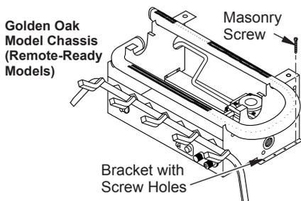
**Figure 14 - Attaching Base Assembly to Fireplace Floor (Remote Ready Models Only)**
