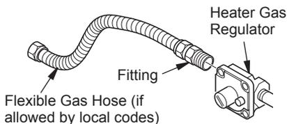
**Figure 11 - Attaching Flexible Gas Hose to Heater Gas Regulator (Variable Manually-Controlled Models Only)**
