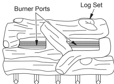
Figure 22 - Installing Vintage Oak Log Sets (Top View)
