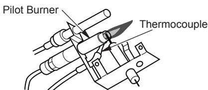
**Figure 38 - Correct Pilot Flame Pattern**
