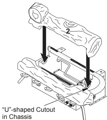
**Figure 27 - Installing Golden Oak 5-Piece Log Set - Log 2**
