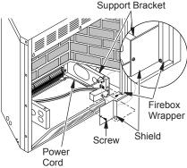
Figure 15 - Installing Shield to Support
