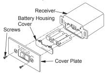
Figure 35 - Battery Install Remote Control Receiver
