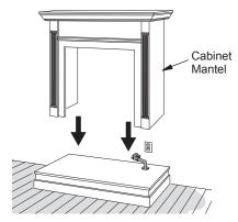
Figure 10 - Installing Cabinet Mantel
