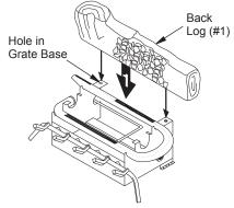
Figure 29 - Installing Back Log (#1) (Base may vary from illustration)
