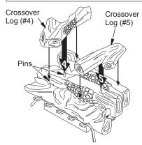
Figure 32 - Installing Crossover Logs (#4 & #5) (Base may vary from illustration)
