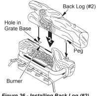
Figure 26 - Installing Back Log (#2) (Base may vary from illustration)
