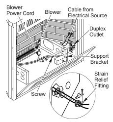
Figure 14 - Connecting Duplex Outlet
