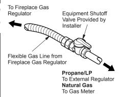
Figure 21 - Attaching Flexible Gas Lines Together
