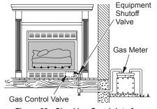
Figure 23 - Checking Gas Joints for Natural Gas
