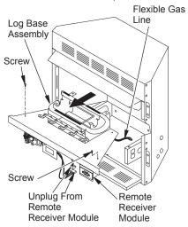
Figure 20 - Removing Log Base Assembly From Fireplace
