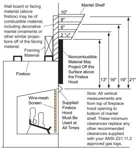
Figure 17 - Minimum Mantel Clearances for Built-In Installation
