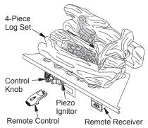
Figure 1 - Log Base Assembly (LMFP33PR Shown)
