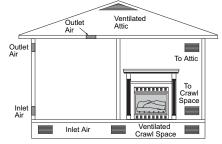
Figure 4 - Ventilation Air from Outdoors
