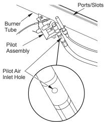
Figure 52 - Pilot Inlet Air Hole
