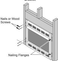
Figure 16 - Attaching Fireplace to Wall Studs
