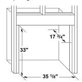
Figure 12 - Rough Opening for Installing in Wall
