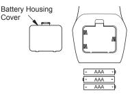
Figure 33 - Battery Install Hand-Held Remote Control
