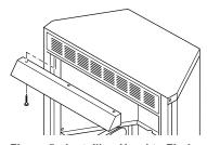
Figure 5 - Installing Hood to Firebox ASSEMBLING AND ATTACHING BLACK TRIM
