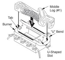
Figure 25 - Installing Middle Log (#1) (Base may vary from illustration)
