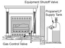
Figure 24 - Checking Gas Joints for Propane/LP Gas
