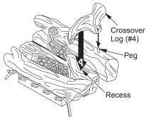
Figure 28 - Installing Crossover Log (#4) (Base may vary from illustration)
