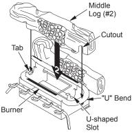
Figure 30 - Installing Middle Log (#2) (Base may vary from illustration)
