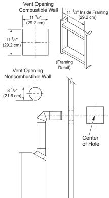
Figure 9 - Vent Opening Requirements
