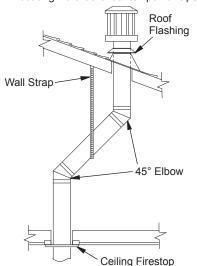
Figure 19 - Offset with Wall Strap and 45° Elbows
