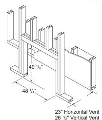
Figure 4 - Framing Clearances for
