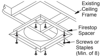
**Figure 10 - Firestop Spacer with Living Space Above Ceiling**
