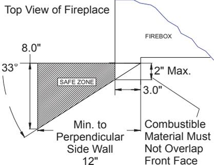
**Figure 4 - Mantel Clearances to Combustible Material**
