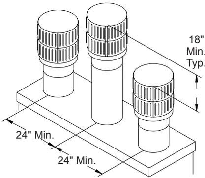
**Figure 16 - Multiple Chase Installation**
