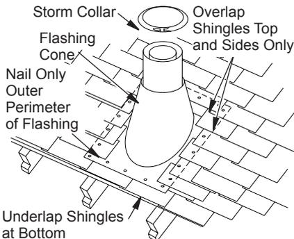
**Figure 13 - Flashing Installation**
