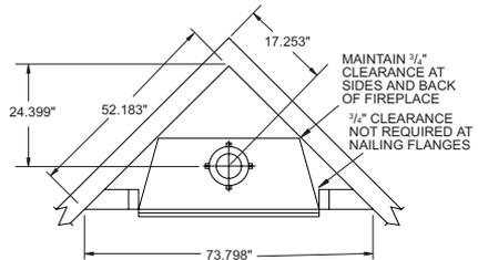
Figure 2 - Corner Installation
