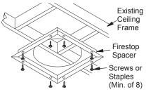
Figure 17 - Firestop Spacer with Living Space Above Ceiling
