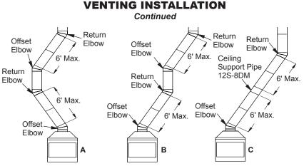
Figure 16 - Typical Offset Terminations (For Systems with 2 Elbow Sets, Maximum Height is 20')
