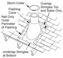
Figure 18 - Flashing Installation
