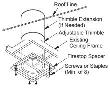
Figure 11 - Attaching Firestop/Thimble Assembly to Ceiling
