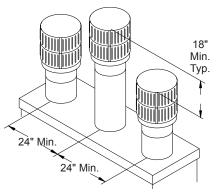
Figure 21 - Multiple Chase Installation
