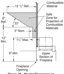
Figure 26 - Mantel Clearances to Combustible Material
