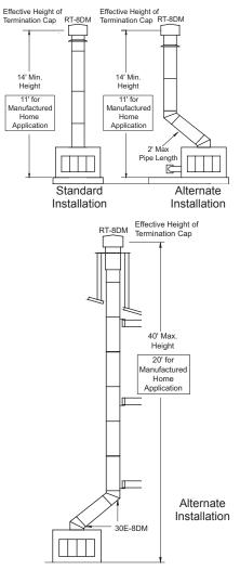
Figure 3 - Standard and Alternate Venting Installation
