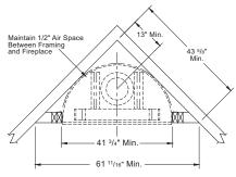
Figure 2 - Corner Installation
