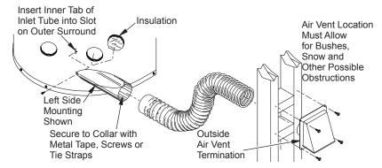
Figure 8 - Outside Air Kit AK6-WE Installation
