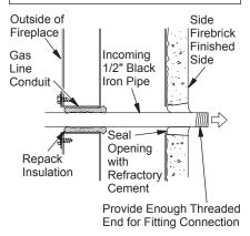
Figure 25 - Gas Line Installation
