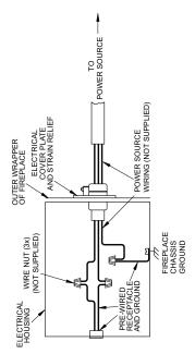
Figure 7 - Fan Kit Wiring Diagram
