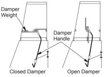
Figure 30 - Damper Operation
