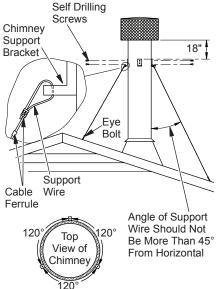
Figure 23 - Support Wires
