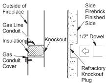
Figure 24 - Gas Line Knockout
