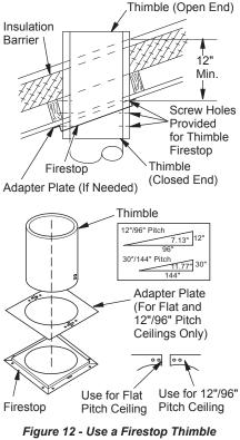
Figure 12 - Use a Firestop Thimble Assembly for Cathedral Ceiling, Insulation Barrier and Roof
