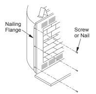
Figure 4 - Nailing Flanges
