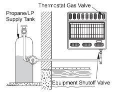
Figure 18 - Checking Gas Joints for Propane/LP Gas
