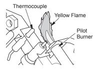
Figure 24 - Incorrect Pilot Flame Pattern
