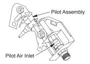
Figure 27 - Pilot Inlet Air (Propane/LP Pilot Shown)
