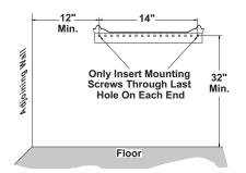
Figure 8 - Mounting Bracket Clearances
