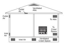
Figure 3 - Ventilation Air from Outdoors
