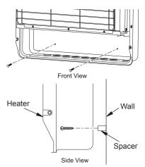
Figure 12 - Installing Bottom Mounting Screws
