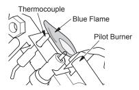
Figure 23 - Correct Pilot Flame Pattern
