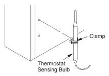
Figure 5 - Attaching Thermostat Sensing
