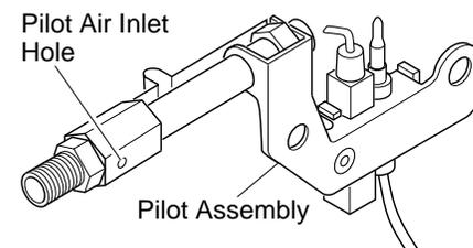
Figure 22 - Pilot Inlet Air Hole
