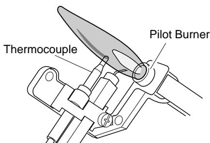
Figure 18 - Correct Pilot Flame Pattern
