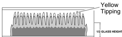
Figure 21 - Incorrect Burner Flame Pattern
