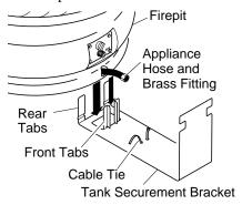
Figure 2 - Attaching Tank Securement Bracket and Cable Tie
