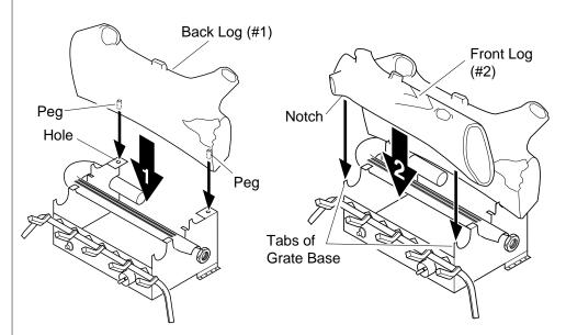
Figure 17 - Installing Back Log
