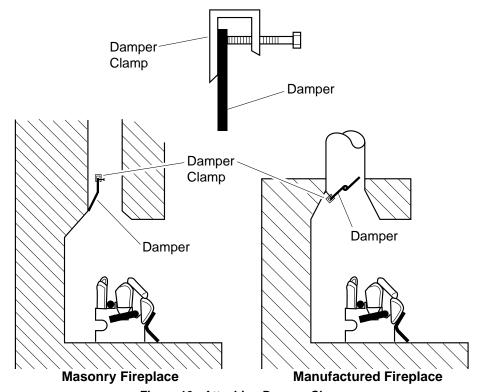
Figure 10 - Attaching Damper Clamp
