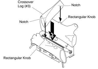
Figure 19 - Installing Crossover Log
