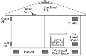
Figure 3 - Ventilation Air from Outdoors
