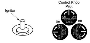
Figure 22 - Ignitor and Control Knob
