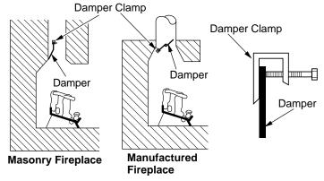
Figure 5 - Attaching Damper Clamp
