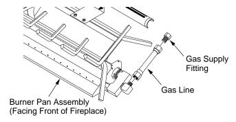
Figure 10 - Connecting Gas to Appliance
