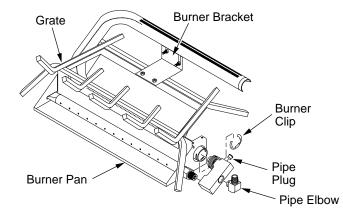
Figure 9 - Installing Burner
