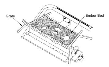
Figure 18 - Installing Ember Bed
