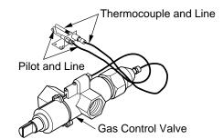
Figure 12 - Gas Control Valve with Thermocouple and Pilot
