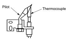
Figure 23 - Thermocouple and Pilot
