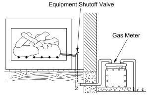
Figure 7 - Checking Gas Joints
