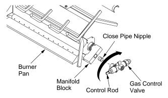
Figure 11 - Installing Gas Control Valve
