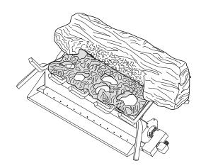
Figure 19 - Installing Back log
