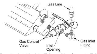
Figure 13 - Installing Inlet Fitting and Gas Connector Tube
