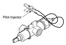
Figure 17 - Installing Propane/LP Pilot Orifice
