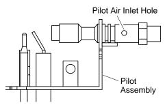
Figure 28 - Pilot Inlet Air Hole
