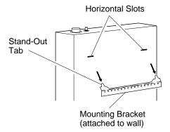
Figure 14 - Mounting Heater Onto Mounting Bracket
