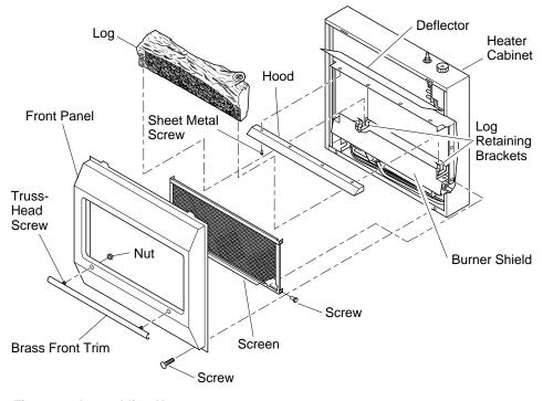
Figure 3 - Assembling Heater
