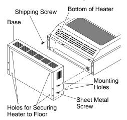
Figure 16 - Attaching Heater to Hearth Base
