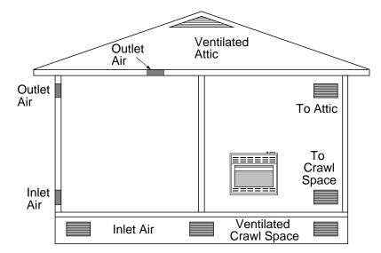
Figure 8 - Ventilation Air from Outdoors
