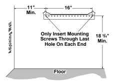
Figure 11 - Mounting Bracket Clearances
