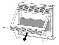
Figure 2 - Removing Front Panel of Heater
