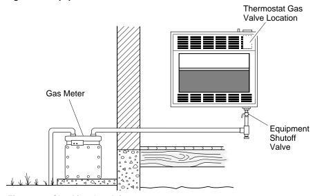
Figure 20 - Checking Gas Joints
