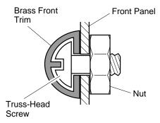
Figure 4 - Attaching Brass Front Trim to Front Panel
