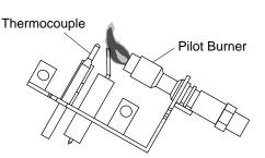
Figure 24 - Incorrect Pilot Flame Pattern
