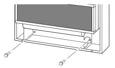
Figure 15 - Installing Bottom Mounting Screws
