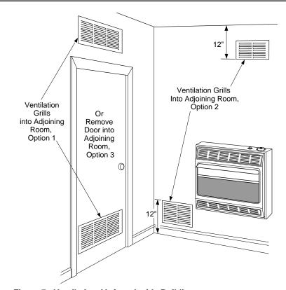
Figure 7 - Ventilation Air from Inside Building
