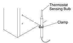
Figure 10 - Attaching Thermostat Sensing Bulb
