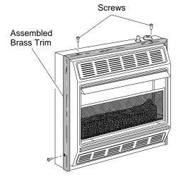
Figure 6 - Attaching Brass Trim to Heater
