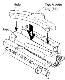
Figure 19 - Installing Crossover Log (#4)
