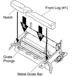
Figure 16 - Installing Front Log (#1)
