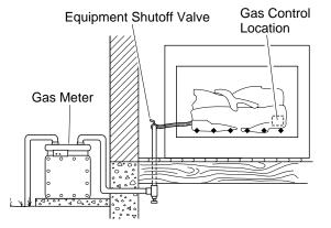
Figure 15 - Checking Gas Joints
