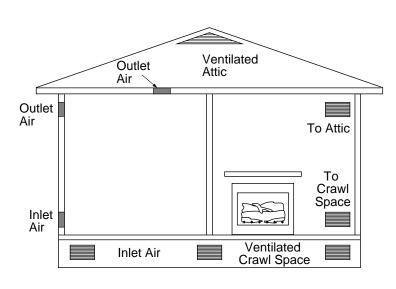
Figure 3 - Ventilation Air from Outdoors
