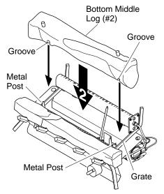
Figure 17 - Installing Bottom Middle Log (#2)
