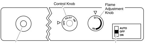
Ignitor Button 5 Figure 21 - Control Knob and Ignitor Button Location
