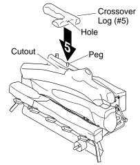
Figure 20 - Installing Crossover Log (#5)
