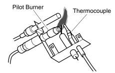
Figure 26 - Incorrect Pilot Flame Pattern
