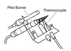
Figure 25 - Correct Pilot Flame Pattern
