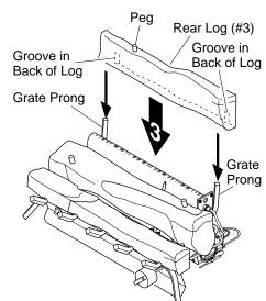
Figure 18 - Installing Rear Log (#3)
