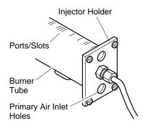
Figure 27 - Injector Holder On Outlet Burner Tube
