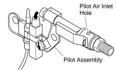
Figure 28 - Pilot Inlet Air Hole
