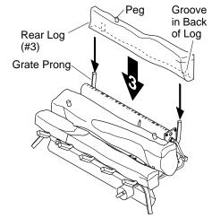
Figure 18 - Installing Rear Log (#3)
