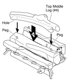
Figure 19 - Installing Top Middle Log (#4)
