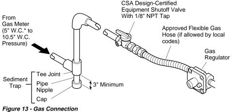
\* Minimum inlet pressure for purpose of input adjustment.
