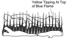
Figure 26 - Incorrect Front Burner Flame Pattern
