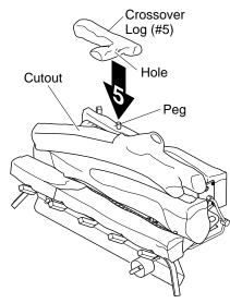
Figure 20 - Installing Crossover Log (#5)
