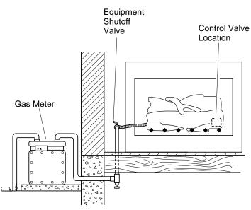
Figure 15 - Checking Gas Joints
