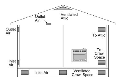
Figure 9 - Ventilation Air from Outdoors
