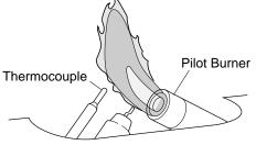
Figure 27 - Incorrect Pilot Flame Pattern
