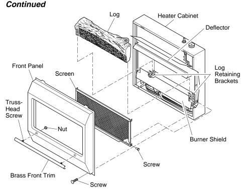
Figure 4 - Assembling Heater
