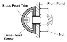
Figure 5 - Attaching Brass Front Trim to Front Panel
