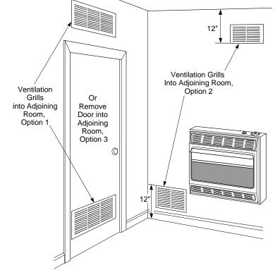
Figure 8 - Ventilation Air from Inside Building
