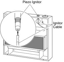
Figure 3 - Attaching Ignitor Cable to Piezo Ignitor
