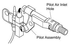
Figure 30 - Pilot Inlet Air Hole
