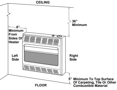
Figure 10 - Mounting Clearances As Viewed From Front of Heater
