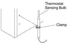
Figure 11 - Attaching Thermostat Sensing Bulb
