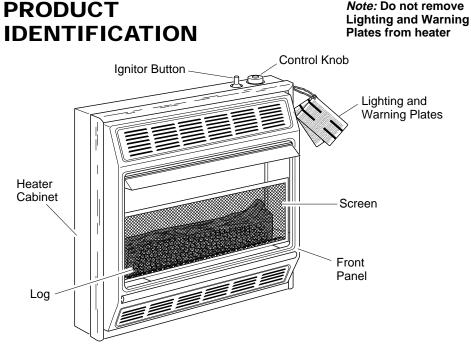
Figure 1 - Vent-Free Gas Log Propane/LP Gas Space Heater
