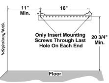
Figure 13 - Mounting Bracket Clearances
