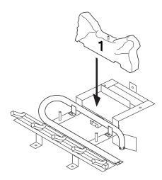
Figure 44 - Installing Log No. 1
