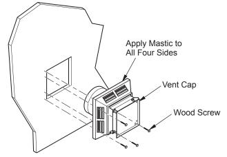
Figure 10 - Installing Horizontal Vent Cap
