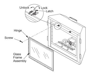
Figure 41 - Removing/Replacing Glass Door
