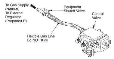
Figure 32 - Attaching Flexible Gas Line to Control Valve
