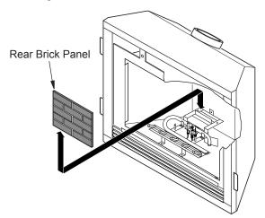
Figure 42 - Installing Rear Brick Panel
