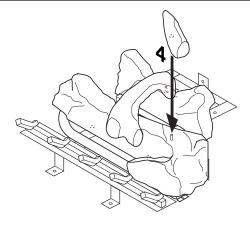
Figure 47 - Installing Log No. 4
