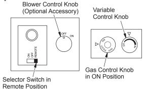
Figure 51 - Setting the Selector Switch, Gas Control Knob and Variable Contorl Knob for Remote Operation
