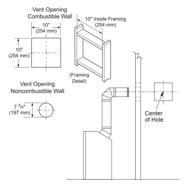
Figure 9 - Vent Opening Requirements
