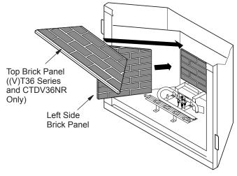
Figure 43 - Installing Left Side and Top Brick Panels
