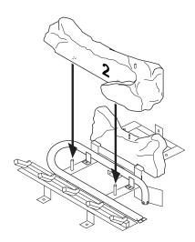
Figure 45 - Installing Log No. 2
