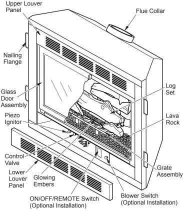
Figure 1 - Tudor Direct-Vent Fireplace with Millivolt Ignition
