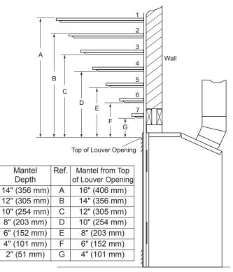
Figure 6 - Clearances for Combustible Mantels
