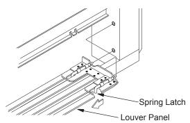
Figure 40 - Removing Louver Panel
