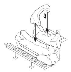
Figure 46 - Installing Log No. 3
