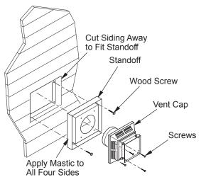
Figure 11 - Installing Siding Standoff
