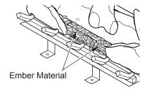
Figure 49 - Placing Ember Material on Burner
