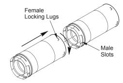
Figure 8 - Vent Pipe Connections
