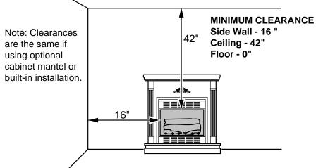
Figure 7 - Minimum Clearance to Wall and Ceiling
