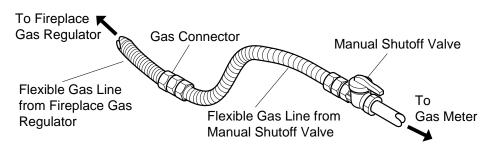
Figure 18 - Attaching Flexible Gas Lines Together
