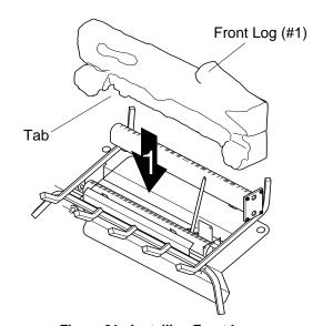
Figure 21 - Installing Front Log
