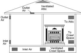
Figure 4 - Ventilation Air from Outdoors
