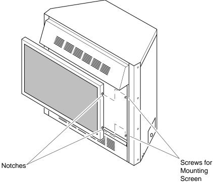
Figure 24 - Installing Fireplace Screen
