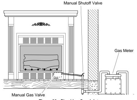
Figure 20 - Checking Gas Joints
