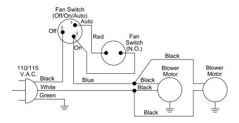
Figure 33 - Blower Wiring Diagram for Thermostat-Controlled Models
