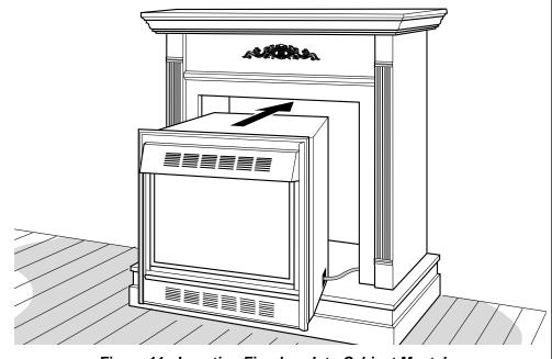
Figure 11 - Inserting Fireplace Into Cabinet Mantel
