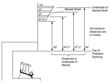
Figure 15 - Minimum Mantel Clearances for Built-In Installation
