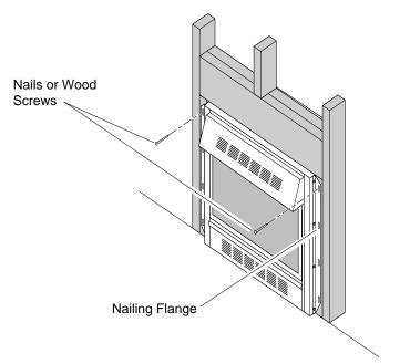
Figure 14 - Attaching Fireplace to Wall Studs
