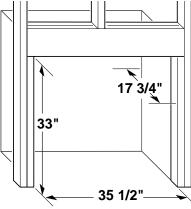
Figure 12 - Rough Opening for Installing in Wall
