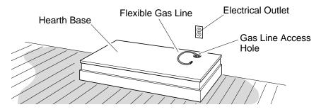
Figure 9 - Placing Hearth Base Accessory Against Wall
