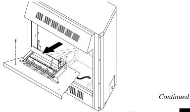
Figure 17 - Removing Log Base Assembly From Fireplace
