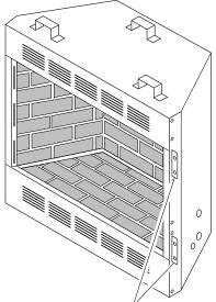
Nailing Flanges Figure 11 - Location of Nailing Flanges (Two on Each Side)
