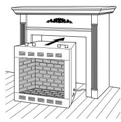
Figure 12 - Inserting Firebox Into Cabinet Mantel
