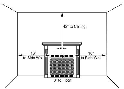
Figure 6 - Minimum Clearance to Wall, Ceiling, and Floor
