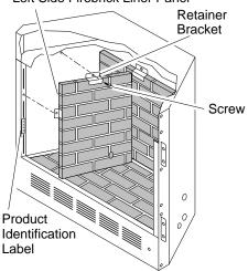
Figure 15 - Removing Side Panel
