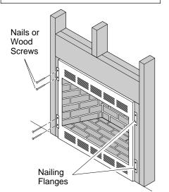
Figure 9 - Attaching Firebox to Wall Studs
