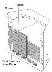
Figure 16 - Removing Rear Firebrick Liner Panel
