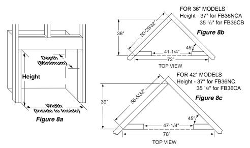
Figure 8 - Rough Opening for Installing in Wall
