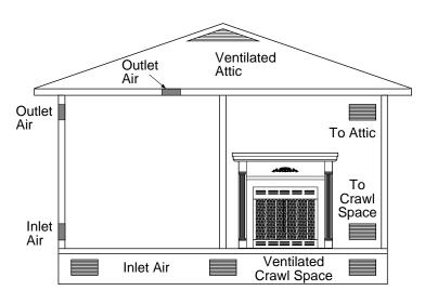
Figure 5 - Ventilation Air from Outdoors
