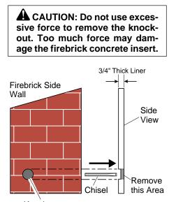
Knockout Figure 14 - Location of Knockout for Gas Line
