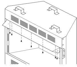
Figure 21 - Screw and Hood Placement for Hood
