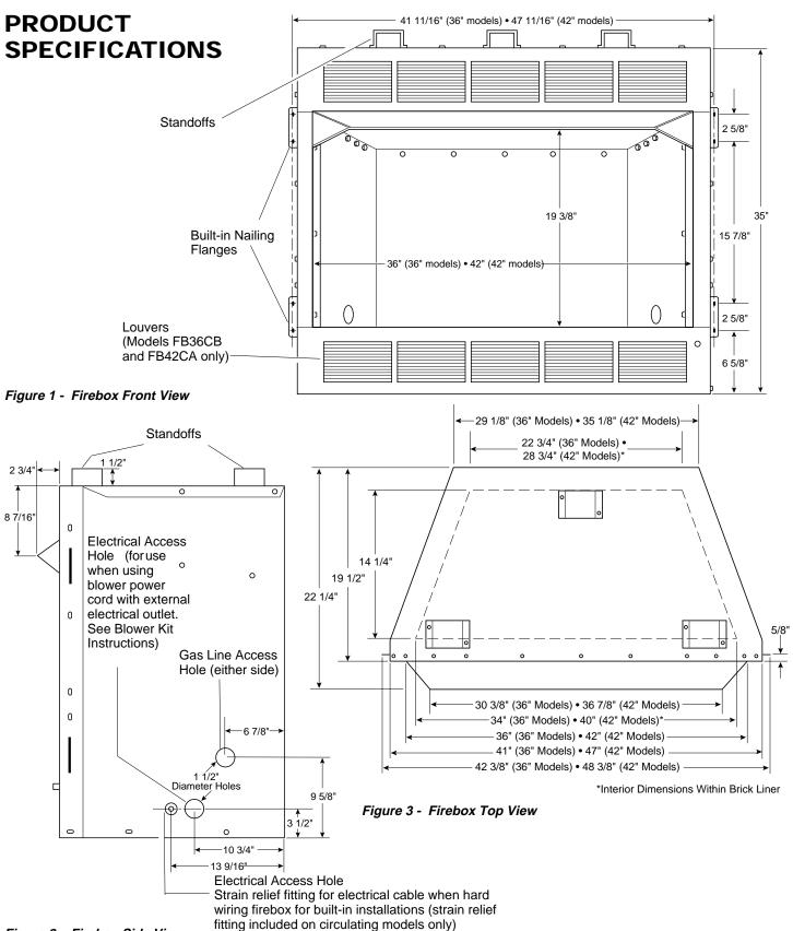
Figure 2 - Firebox Side View
