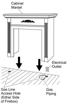
Figure 10 - Installing Cabinet Mantel
