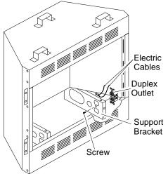
Figure 19 - Removing Duplex Outlet
