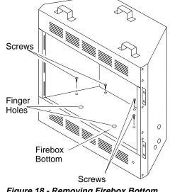
Figure 18 - Removing Firebox Bottom
