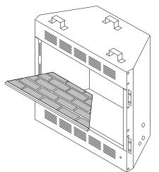
4. Remove the four Phillips screws in firebox bottom.
