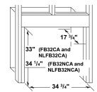
Figure 16 - Rough Opening for Installing in Wall
