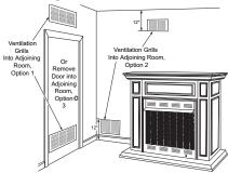
Figure 4 - Ventilation Air from Inside Building
