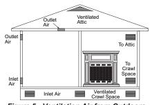
Figure 5 - Ventilation Air from Outdoors
