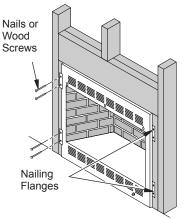
Figure 18 - Attaching Firebox to Wall Studs
