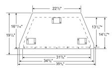
\*Note: 14 <sup>1</sup>/<sub>4</sub>" is total firebox cavity depth including brick liner. 13 <sup>1</sup>/<sub>4</sub>" is depth of flat floor including brick liner.
