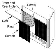
Figure 15 - Installing Fireplace Screen (Shown Without Fireplace Hood for Clarity)
