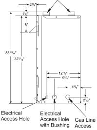
Figure 2 - Firebox Side View
