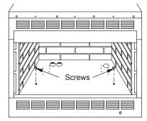
Figure 8 - Removing Screws from Firebox Bottom
