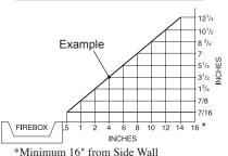
Figure 6 - Minimum Clearance for Combustible to Wall
