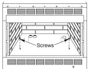
Figure 13 - Removing Firebox Bottom
