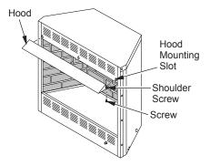
Figure 14 - Installing Fireplace Hood
