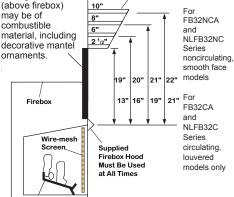
Figure 7 - Minimum Mantel Clearances for Built-In Installation
