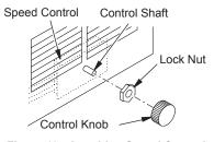
Figure 10 - Attaching Speed Control
