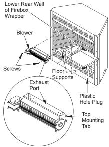
Figure 9 - Mounting Blower to Firebox
