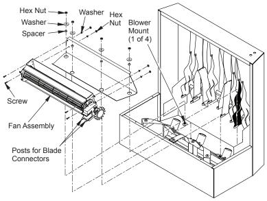
Figure 35 - Removing Fan Assembly (Shown without Firebox for Clarity)
