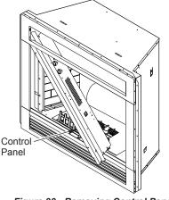
Figure 30 - Removing Control Panel
