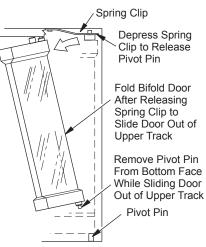
Figure 12 - Installing/Removing Glass Doors
