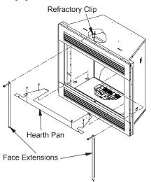
Figure 32 - Removing Hearth Pan and Face Extensions (Extensions for E32 Series Only)
