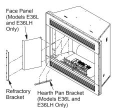
Figure 16 - Removing Refractory Bracket and Hearth Pan Bracket
