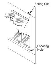
Figure 14 - Installing Fixed Glass Doors
