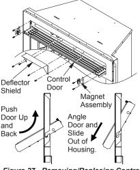
Figure 27 - Removing/Replacing Control Door
