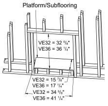
Figure 5 - Framing Dimensions
