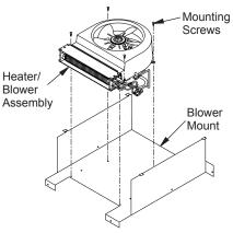
Figure 20 - Mounting Alternate Heater/ Blower
