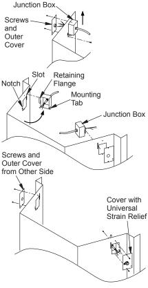
Figure 7 - Relocating Junction Box to Left
