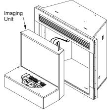
Figure 39 - Removing Imaging Unit
