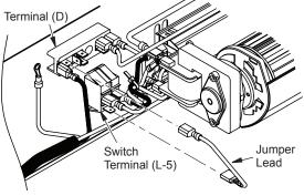
Figure 25 - Connecting Jumper Lead
