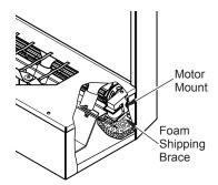
Figure 8 - Removing Shipping Brace
