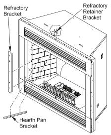
Figure 17 - Installing Brick Panels and Brackets
