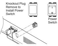
Figure 21 - Installing Heater Power Switch
