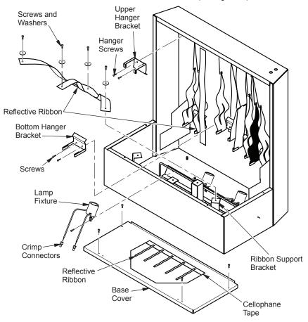
Figure 37 - Replacing Fixtures (Shown without Flrebox for Clarity)
