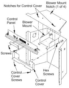
Figure 18 - Disassembling Blower Mount
