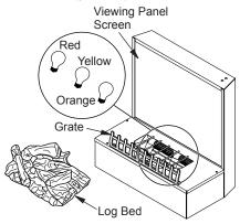
Figure 9 - Bulb Placement
