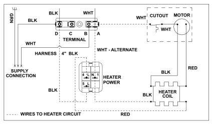
Figure 22 - Heater Circuit Diagrams
