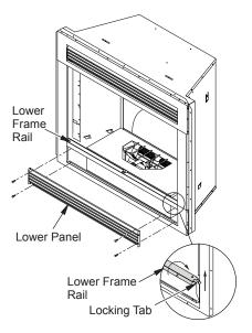
Figure 38 - Removing Lower Louver Panel and Frame Rail
