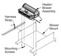
Figure 19 - Mounting Heater/Blower
