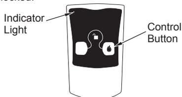
**Figure 54 - On/Off Hand-Held Remote Control Unit HRC100**
