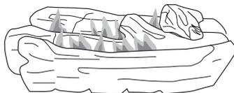
**Figure 49 - Correct Burner Flame Pattern**
