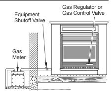
Figure 26 - Checking Gas Joints (Natural Gas Only)
