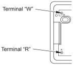
Figure 33 - Thermostat Base Terminals "W" and "R"
