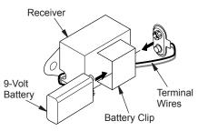
Figure 28 - Attaching Battery to Receiver
