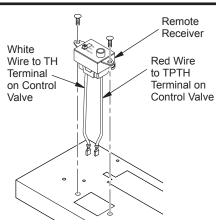
Figure 29 - Installing Remote Receiver
