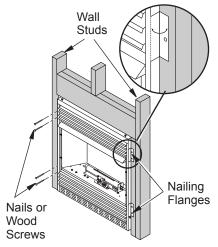
Figure 9 - Attaching Fireplace to Wall Studs
