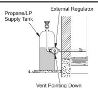
Figure 21 - External Regulator With Vent Pointing Down
