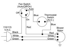
Figure 17 - Wiring Diagram For Blower Accessory Standard Installation
