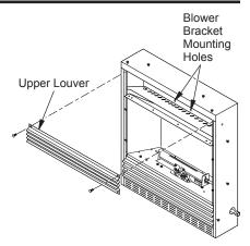
Figure 15 - Removing Upper Louver
