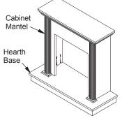
Figure 12 - Installing Cabinet Mantel onto Hearth Base
