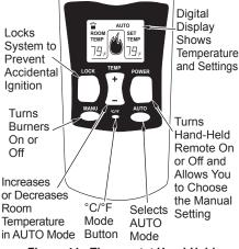
Figure 44 - Thermostat Hand-Held Remote Control Unit
