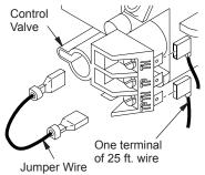
Figure 31 - Connecting Wire Terminals
