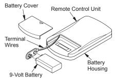
Figure 30 - Installing Battery in Hand-Held Remote Control Unit
