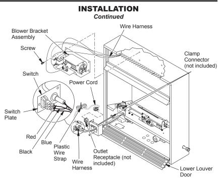
Figure 20 - Installing Blower (Thermostat Unit Shown)
