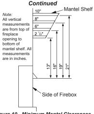
Figure 10 - Minimum Mantel Clearances for Built-In Installation
