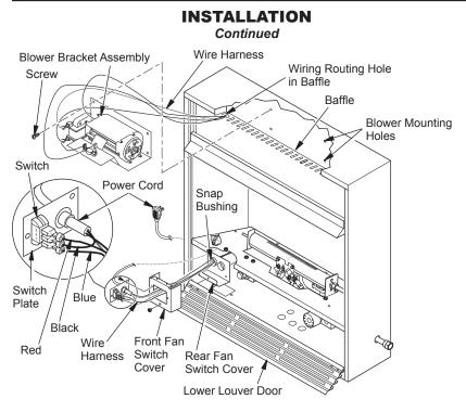
Figure 16 - Installing Blower (Thermostat Unit Shown)
