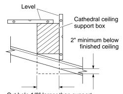
Cut hole 1/8" larger than support box when projected onto roofline
