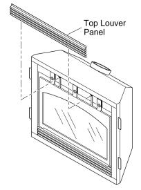
Figure 43 - Removing Top Louver Panel
