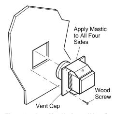
Figure 13 - Installing Horizontal Vent Cap
