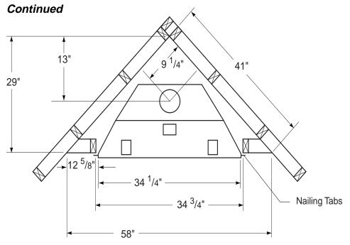
Figure 6 - Framing Clearances for Corner Installation
