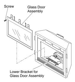
Figure 44- Removing/Replacing Glass Door
