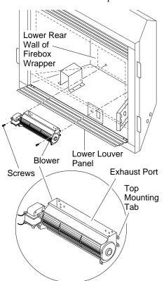
Figure 30 - Mounting Blower to Firebox
