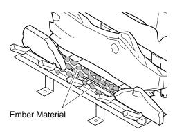
Figure 51 - Placing Ember Material on Burner
