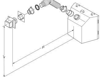
Figure 18 - Horizontal Termination Using Flexible Venting
