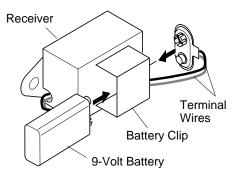
Figure 40 - Attaching Battery to Receiver
