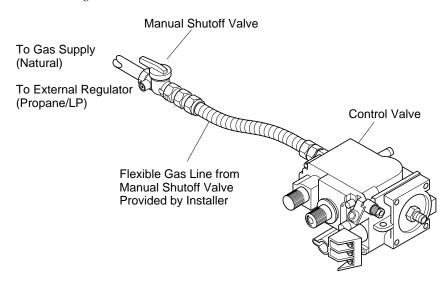
Figure 36 - Attaching Flexible Gas Line to Control Valve
