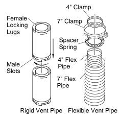
Figure 11 - Vent Pipe Connections
