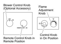
Figure 53 - Setting for Remote Operation
