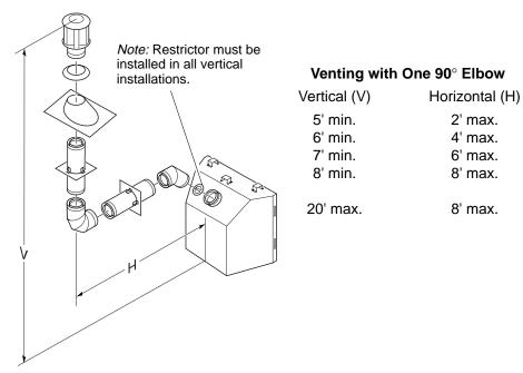
Figure 26 - Vertical Rigid Venting Configuration Using One 90° Elbow
