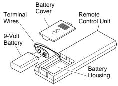
Figure 42 - Installing Battery in Hand-Held Remote Control Unit
