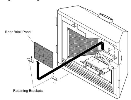
Figure 46 - Installing Rear Brick Panel and Retainer Brackets
