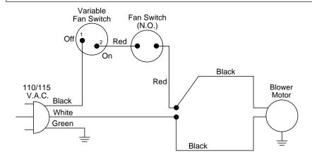
Figure 56 - Blower Wiring Diagram for Thermostat-Controlled Models
