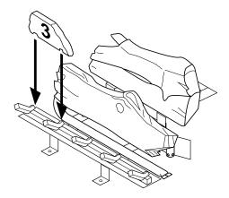
Figure 49 - Installing Log No. 3
