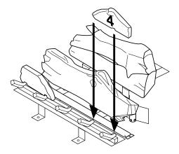
Figure 50 - Installing Log No. 4
