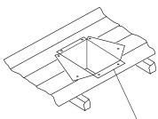
Non-hardening Mastic under all edges of support box before nailing
