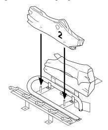
Figure 48 - Installing Log No. 2
