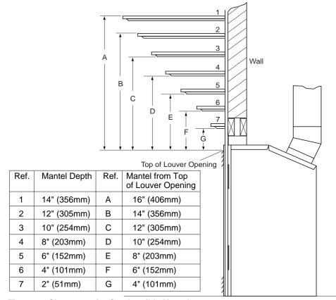
Figure 7 - Clearances for Combustible Mantels
