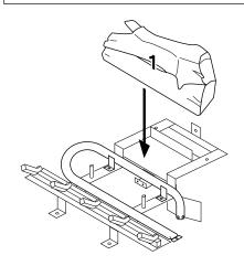
Figure 47 - Installing Log No. 1
