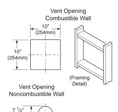
Figure 12 - Vent Opening Requirements
