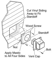
Figure 14 - Installing Vinyl Siding Standoff
