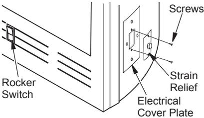
Figure 6 - Fan Kit BK2 Electrical Cover
