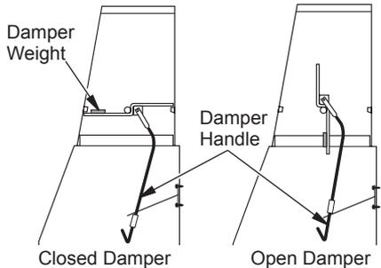
Figure 30 - Damper Operation
