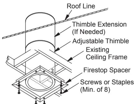
**Figure 11 - Attaching Firestop/Thimble Assembly to Ceiling**
