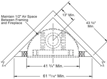
Figure 2 - Corner Installation
