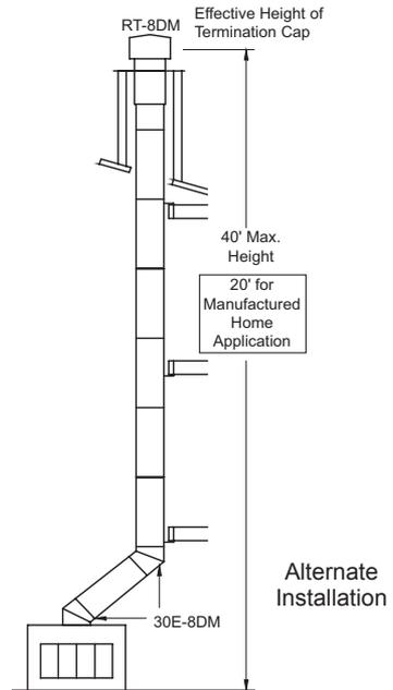
Figure 3 - Standard and Alternate Venting Installation
