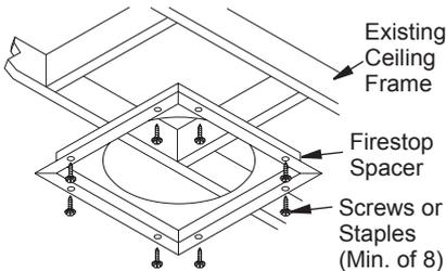
Figure 17 - Firestop Spacer with Living Space Above Ceiling
