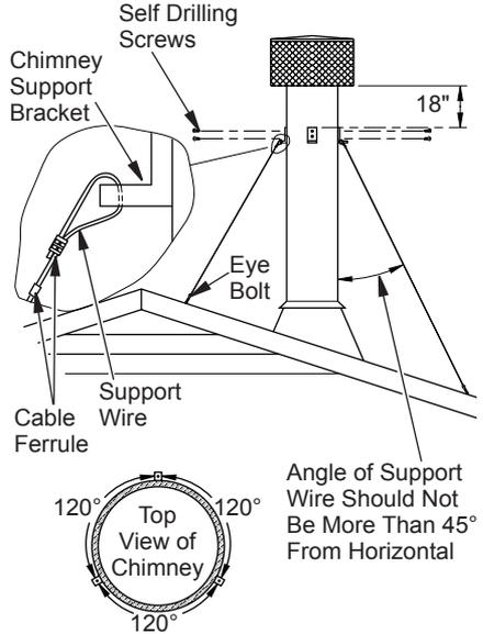
Figure 23 - Support Wires
