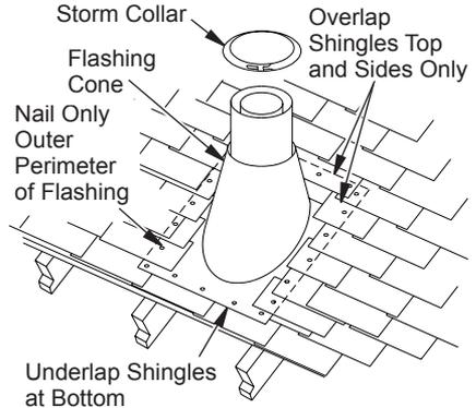
Figure 18 - Flashing Installation
