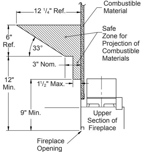
**Figure 26 - Mantel Clearances to Combustible Material**
