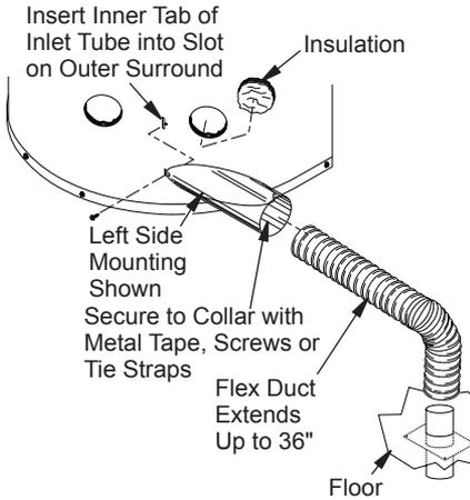
Figure 9 - Outside Air Kit AK6E Installation
