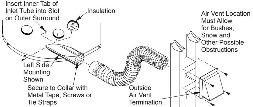
Figure 8 - Outside Air Kit AK6-WE Installation
