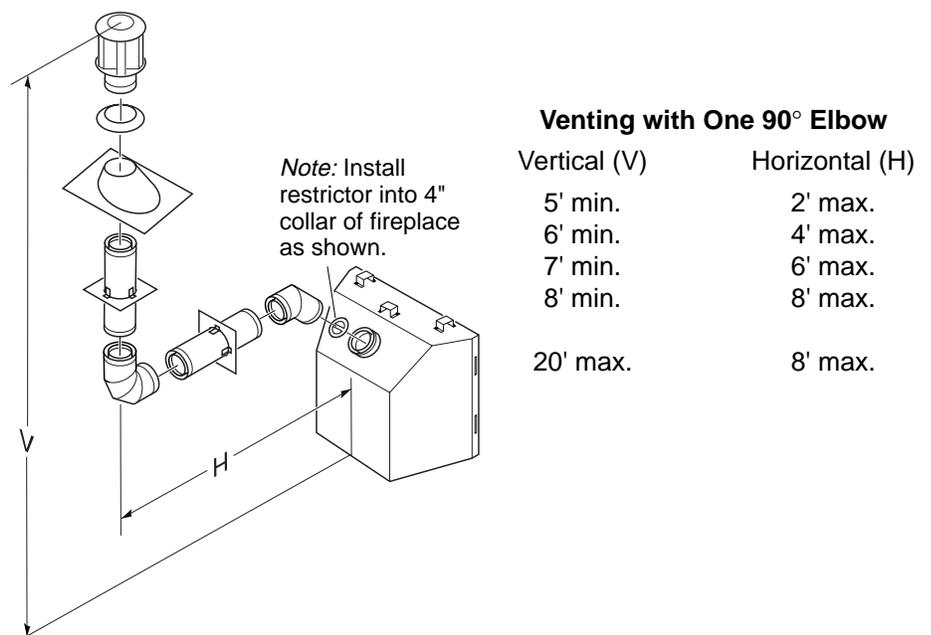
**Figure 26 - Vertical Rigid Venting Configuration Using One 90° Elbow**
