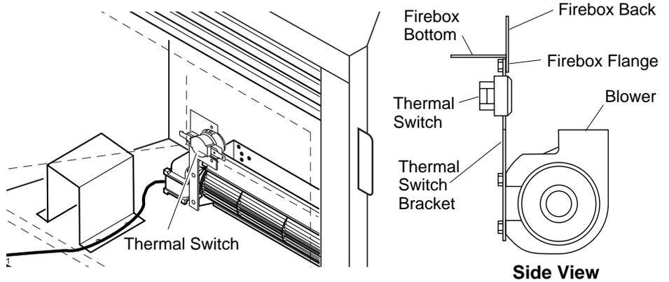
Figure 31 - Locating Thermal Switch Against Back of Firebox
