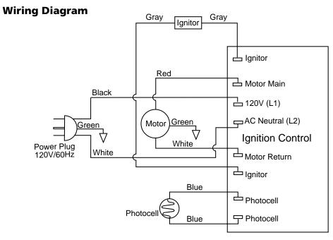
Figure 35 - Wiring Diagram, Models 2E510F and 2E511F
