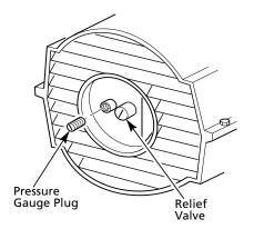
Figure 12 - Pressure Gauge Plug Removal
