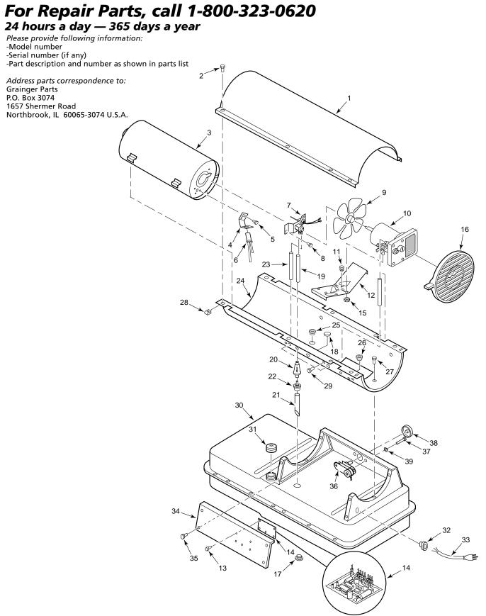
Figure 32 - Repair Parts Illustration for Model 3E218F
