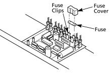
Figure 27 - Replacing Fuse
