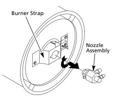
Figure 20 - Removing Nozzle Assembly, All Models
