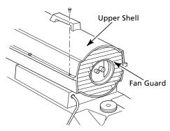
Figure 7 - Upper Shell Removal, Models 2E510F and 2E511F
