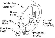
Figure 19 - Removing Air and Fuel Line Hoses (3E218F and 3E219F Btu/Hr Models Only)
