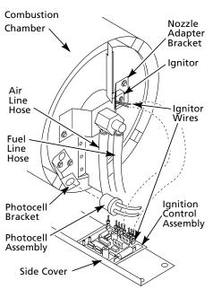
Figure 16 - Disconnecting Ignitor Wires from Ignition Control Assembly
