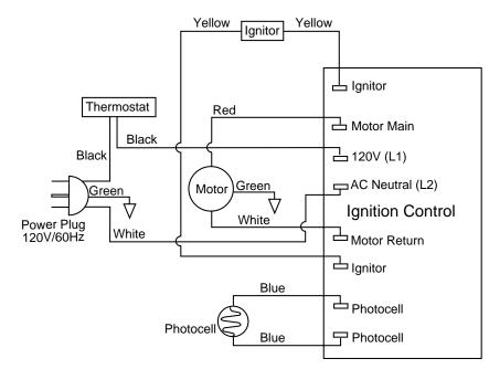
Figure 36 - Wiring Diagram, Models 3E218F and 3E219F
