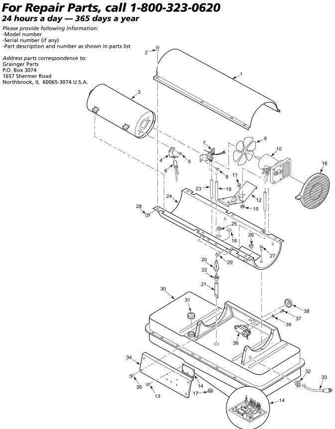
Figure 33 - Repair Parts Illustration for Model 3E219F
