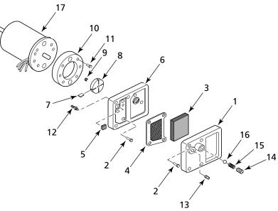
Figure 29 - Burner Head Assembly for All Models
