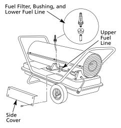
Figure 15 - Fuel Filter Removal, Models 3E218F and 3E219F
