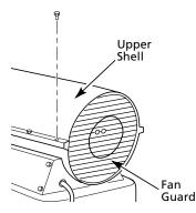
Figure 8 - Upper Shell Removal, Models 3E218F and 3E219F
