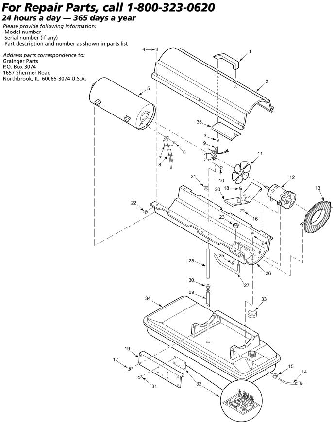
Figure 31 - Repair Parts Illustration for Models 2E510F and 2E511F
