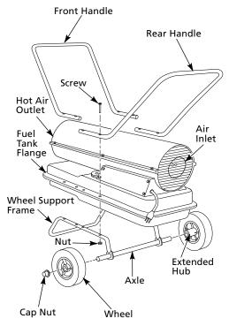
Figure 6 - Wheel and Handle Assembly, Models 3E218F and 3E219F Only **IMPORTANT**: When installing wheels, point extended hub of wheels toward wheel support frame (See Figure 6).
