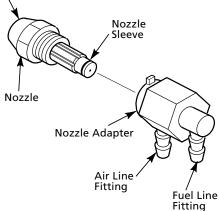
Figure 21 - Nozzle and Nozzle Adapter, All Models
