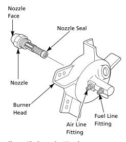
Figure 17 - Removing Nozzle
