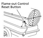
Figure 5 - Flame-out Control Reset Button
