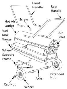
Figure 4 - Wheel and Handle Assembly
