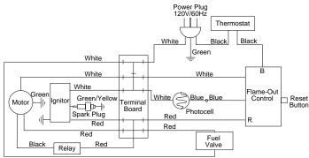
Figure 26 - Wiring Diagram
