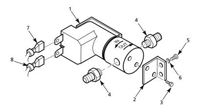
Figure 23 - Fuel Valve Assembly
