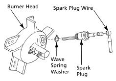
Figure 13 - Spark Plug Removal
