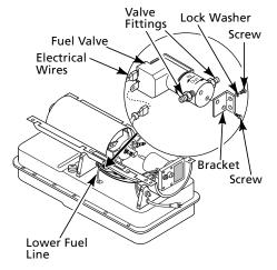
Figure 12 - Fuel Valve Replacement
