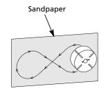
Figure 20 - Sanding Rotor
