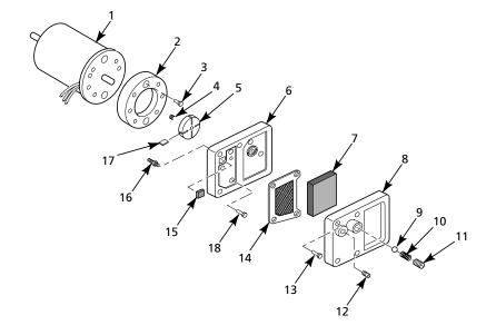
Figure 21 - Motor and Pump Assembly
