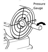
Figure 10 - Adjusting Pump Pressure
