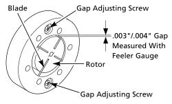
Figure 19 - Gap Adjusting Screw Locations
