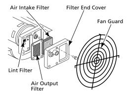
Figure 8 - Air Output, Air Intake, and Lint
