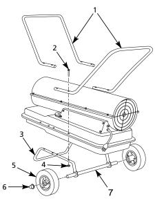
Figure 25 - Handle and Wheel Assembly
