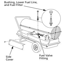
Figure 11 - Fuel Filter Removal
