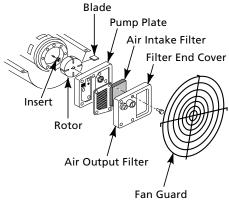
Figure 18 - Rotor Location
