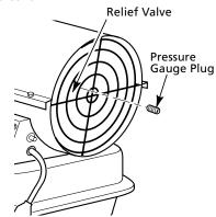
Figure 9 - Pressure Gauge Plug Removal
