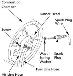
Figure 16 - Removing Burner Head
