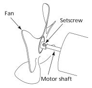
Figure 9 - Fan, Motor Shaft, and Setscrew Location
