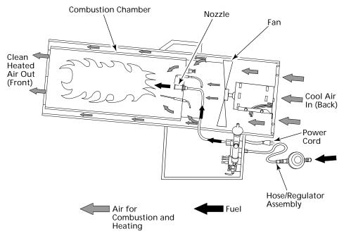
Figure 3 - Cross Section Operational View
