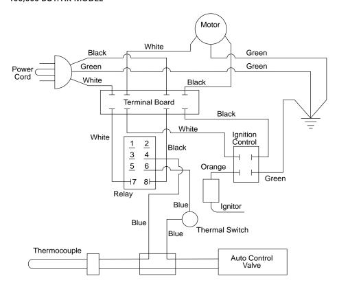
Figure 14 - Electrical Connection Diagram
