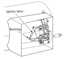
Figure 11 - Removing Ignitor Wire from Spark Transformer
