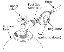
Figure 4 - Regulator With Vent Pointing Down
