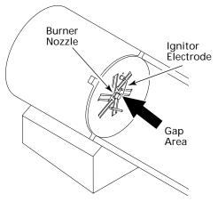
Figure 13 - Clearance between Ignitor Electrode and Target Plate
