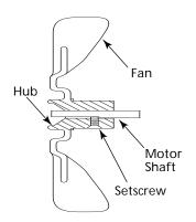
Figure 10 - Fan Cross Section
