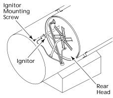
Figure 12 - Removing Ignitor Mounting Screw and Ignitor
